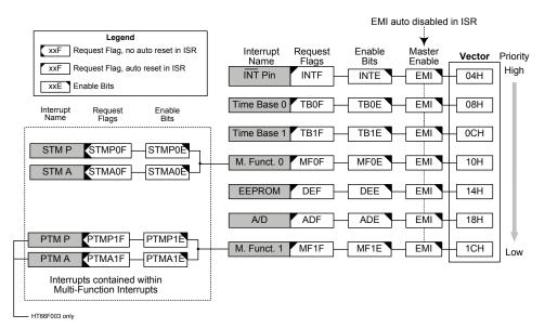
Interrupt Structure - HT66F002/HT66F0025/HT66F003
