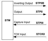
**STM Function Pin Control Block Diagram**
