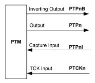
**PTM Function Pin Control Block Diagram**
