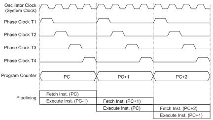
System Clock and Pipelining
